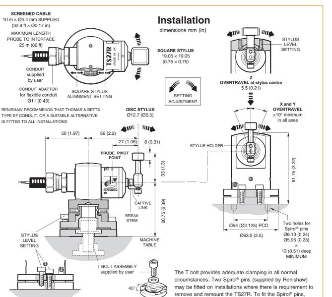
drill two holes in the machine table to correspond with two
