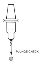
When running the following cycle after machining, the tool is automatically positioned over the laser beam. It is then plunged into the beam to check its overall length. With the following example both long and short tool conditions can be checked to a tolerance of 0.5mm.
