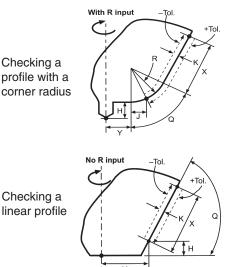
This cycle is used to check the profile of ballnose cutters, cutters with corner radii, and cutters with linear profiles. The profile is checked to find out if it is within a specified form tolerance.
