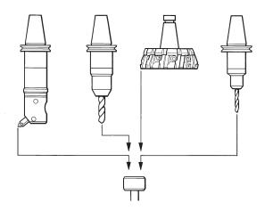
The tool will be selected automatically from the tool change magazine, positioned over the stylus then measure the length / diameter before returning to home position and update the relevant offsets.
